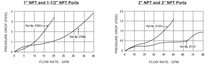
Note: Tests conducted with units in horizontal position (lead wires up) with water at +70°F (21°C).
